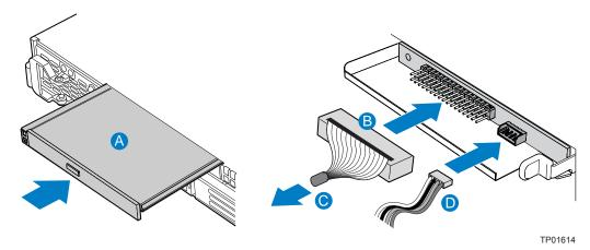
Figure 30. Installing a DVD/CDROM Drive into the Chassis
